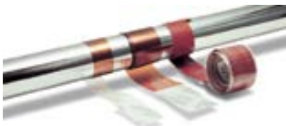
Built-to-order shrink bands are pre-stretched strips of film with adhesive coated ends. Wrap around the heater and heat to shrink. Stretch tape installs quickly with no heat required.
